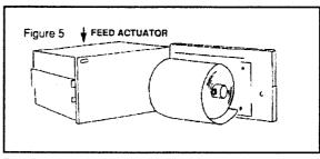
Turn the paper roll so that any loose turns are wound snugly against the roll. Close the printer door.
